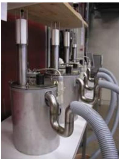
**Figure 2.** CSTR reactors used for treating untreated and autoclaved food waste.
